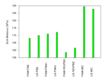
Figure 4. (Color online) The Equilibrium bulk moduli at 0 K (without zero point-energy included) for the different Bi, Ga and O pseudo-potentials employed in this work. We extracted this data from the Murnaghan fit.
