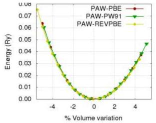
Figure 2. (color on line) Equation of state as a function of percent volume change with respect to theoretical equilibrium configurations for three selected pseudo-potentials. Between -2 and +2, the curves fit each other but small deviations in curves start appearing for higher percentage volumes.
