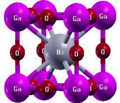
Figure 1. (color on line) the unit cell of simple cubic structure of  $BiGaO_3$
