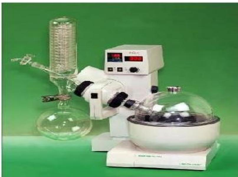
**Plate 3: Rotary evaporator for removing solvent methanol.**
