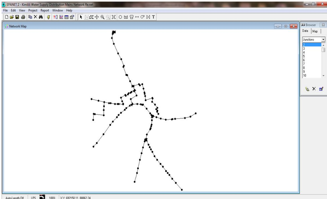
**Figure 4. 10: Kimilili Water Supply EPANET 2.0 pipeline distribution network model with hidden backdrop layer of distribution network.**
