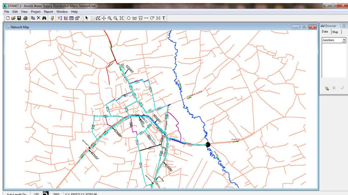
**Figure 4. 8: Kimilili Water Supply EPANET 2.0 backdrop layer of distribution network.**
