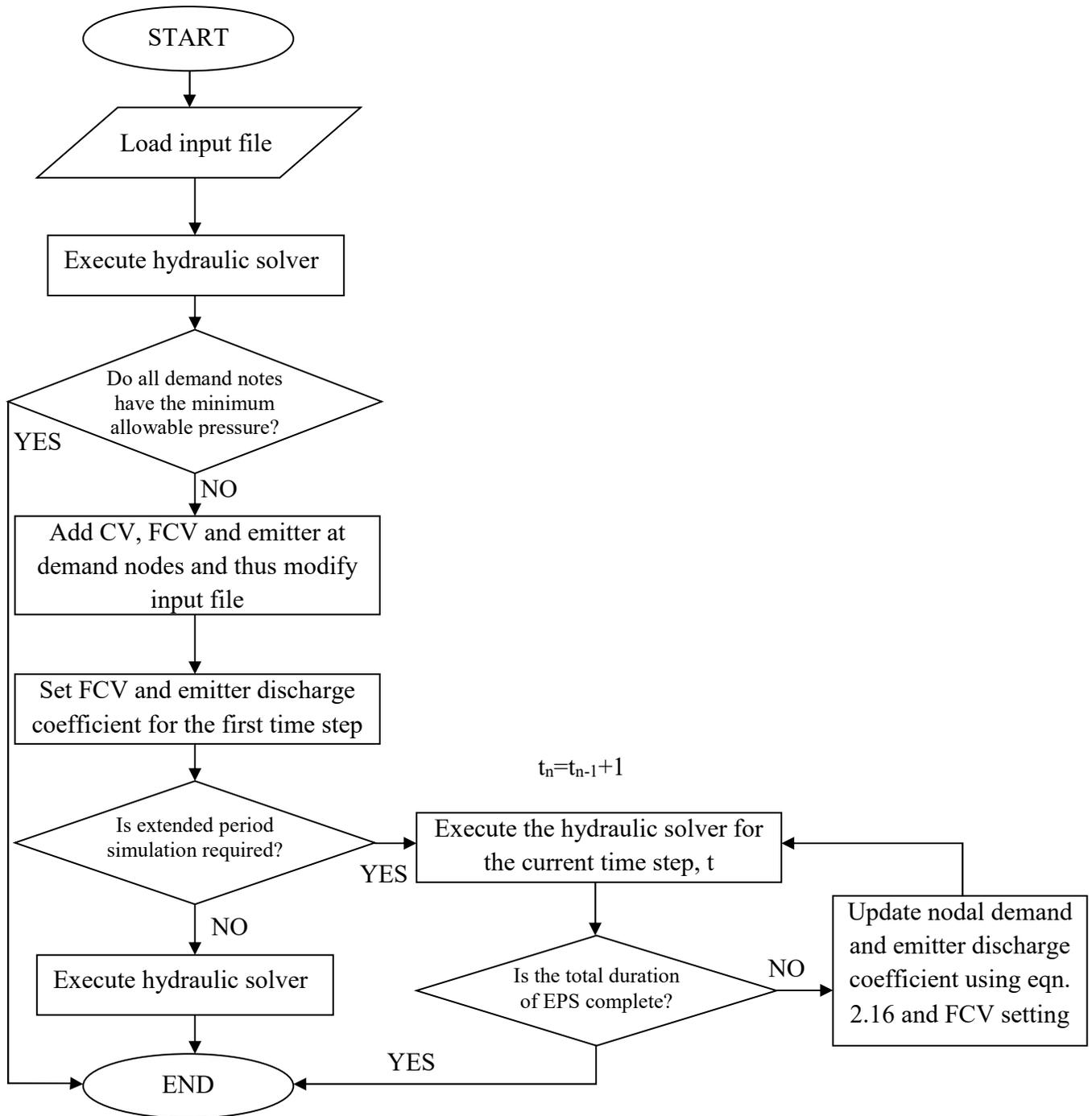
**Figure 3. 3: EPANET pressure dependent analysis algorithm flow chart.**
