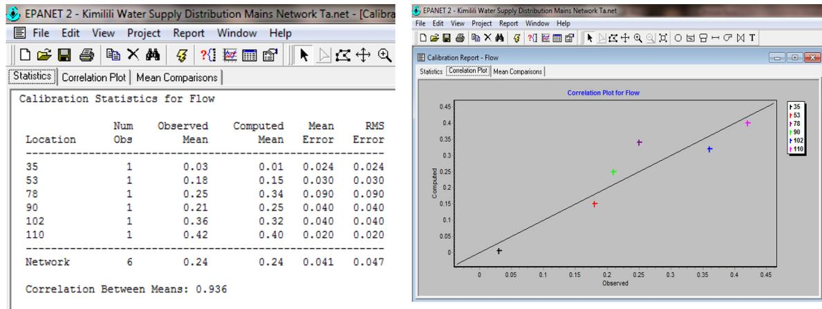
Figure 4. 12: Link Flows Calibration.
