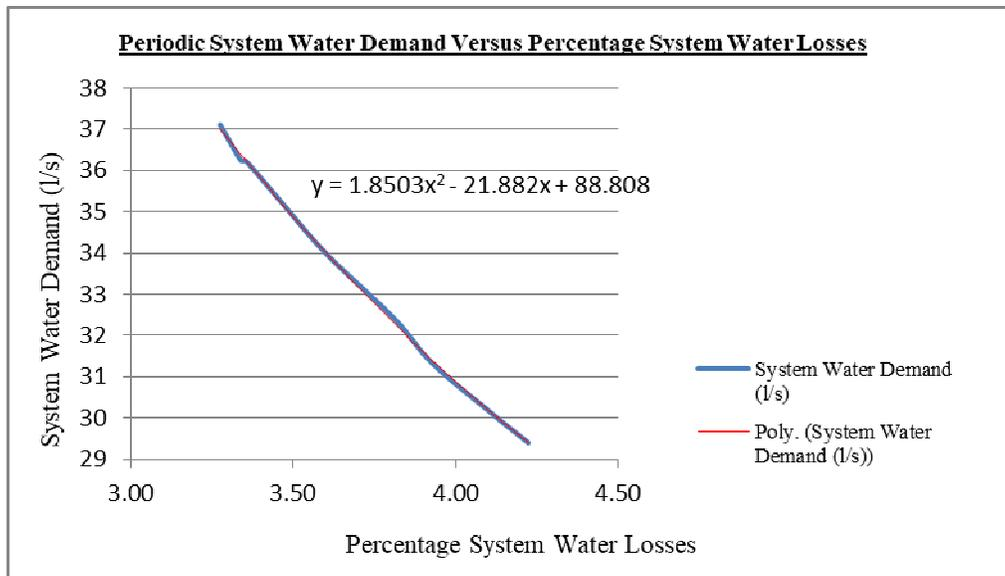
**Figure 4. 19: Mathematical Relationship Between Periodic System Water Demand And Percentage System Water Losses.**
