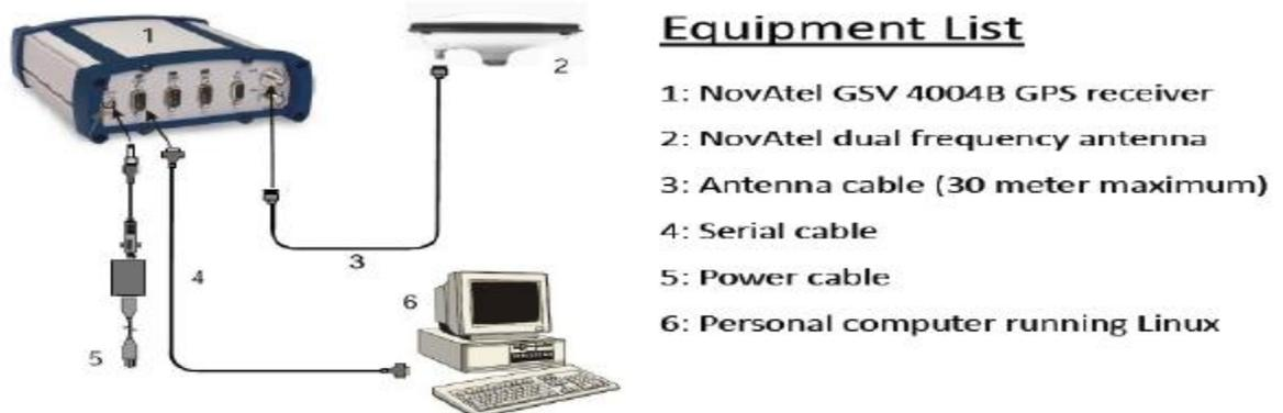
**Figure 3.1: GPS-SCINDA system component (Carrano, 2007)**
