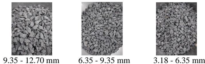
**Figure 3.** Physical images of aggregates
