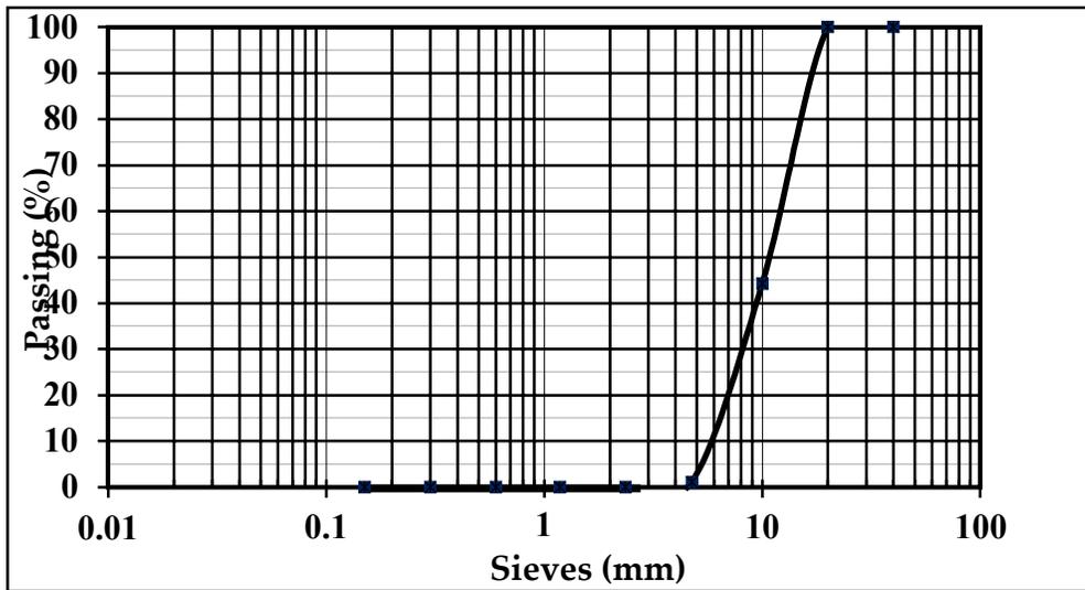
**Figure 3. 2: Grading Curve for coarse Aggregates**
