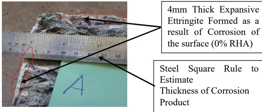
**Figure 4. 9: Corrosion Depth for Sample with 0% RHA and 0.4 W/C**
