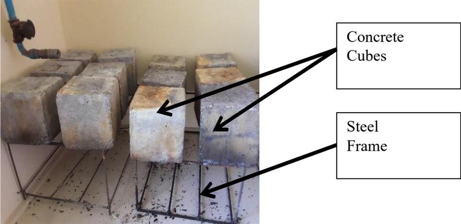
**Figure 3. 8: Samples air dried after exposure in acidic solution.**
