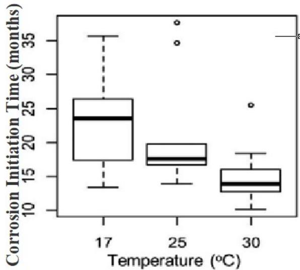
**Figure 2. 1: Relationship between temperature and corrosion initiation time (Guangming, 2014)**
