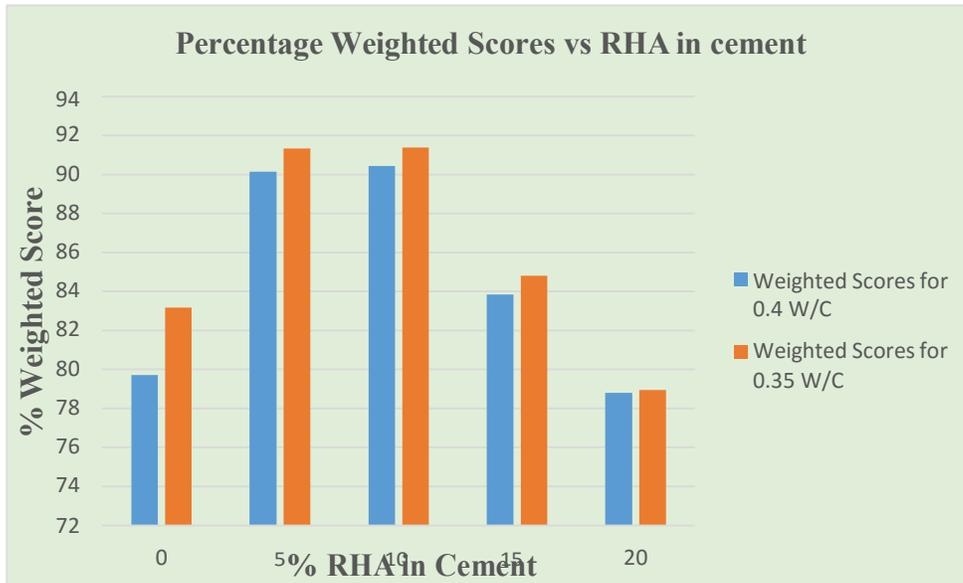
**Figure 4. 11: Weighted Scores for Different % RHA in Cement**
