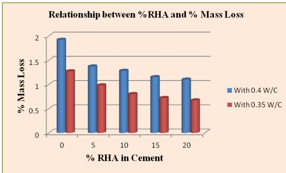
Figure 4. 7: Comparison of % Mass Loss for the two W/C Ratios
