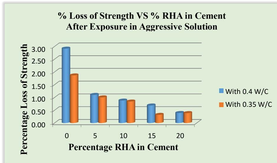
**Figure 4. 4: Percentage Loss of Strength vs % RHA in Cement**
