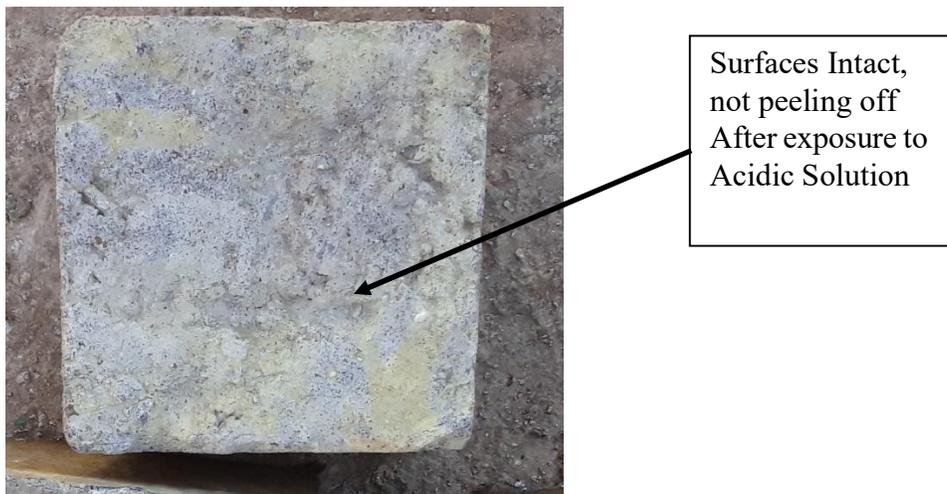
**Figure 4. 6: Sample with 20% RHA and 0.35 W/C ratio,**
