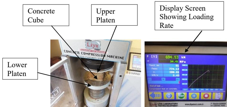
Figure 3. 9: Compression Test on Samples
