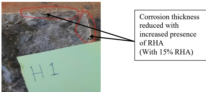
**Figure 4. 10: Corrosion Depth for Sample with 15% RHA and 0.35 W/C**
