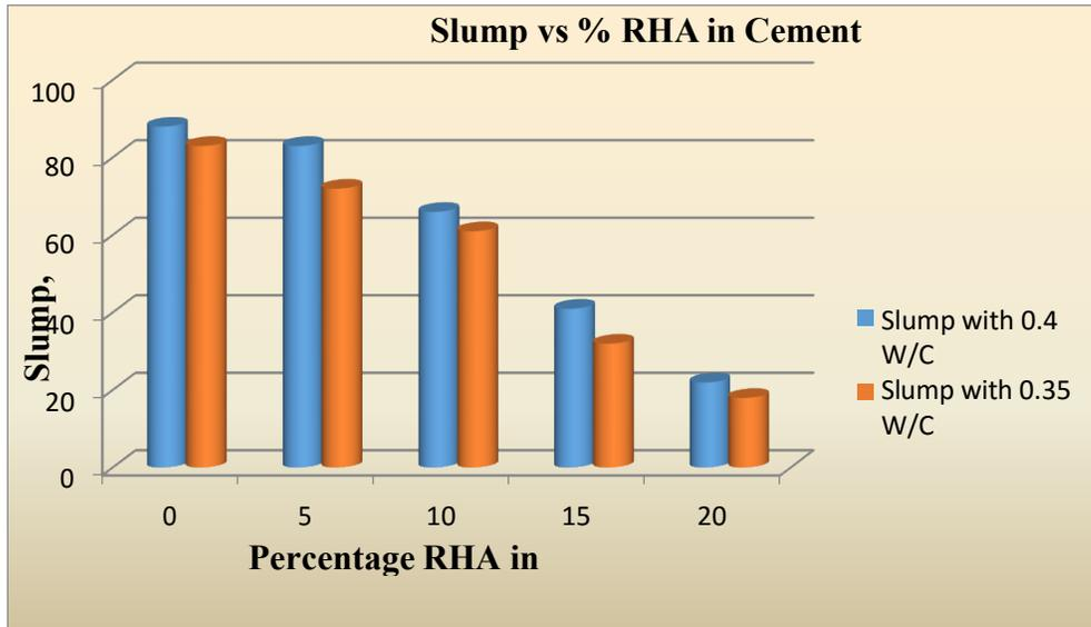
**Figure 4. 1: Slump Test Results for Fresh Concrete**
