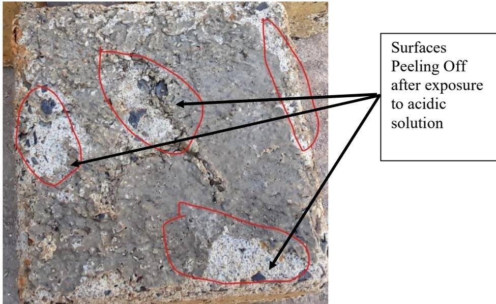
**Figure 4. 5: Sample with 0% RHA showing surface degradation after exposure to acidic solution**
