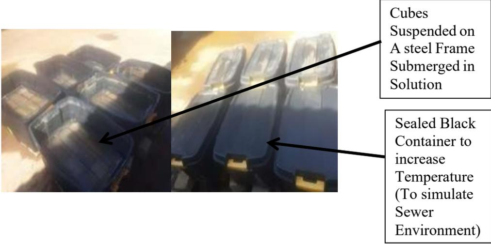
**Figure 3. 7: Samples in acidic solution**
