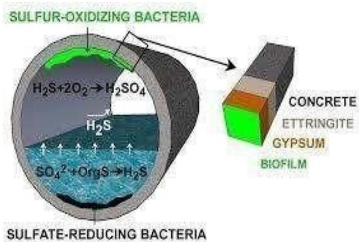
**Figure 1. 3: Corrosion Process in a sewer (Wells, 2009)**
