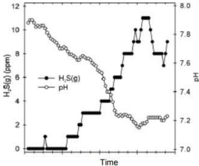
**Figure 2. 2: Correlation linking sewage pH and the level of H<sub>2</sub>S (Nielsen, 2006).**
