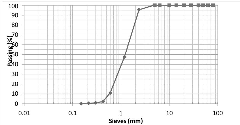
**Figure 3. 3: Grading Curve for fine Aggregates**
