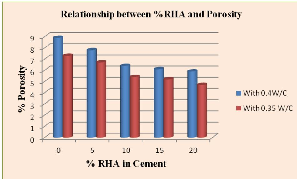
**Figure 4. 8: Comparison of % Porosities of degraded samples**
