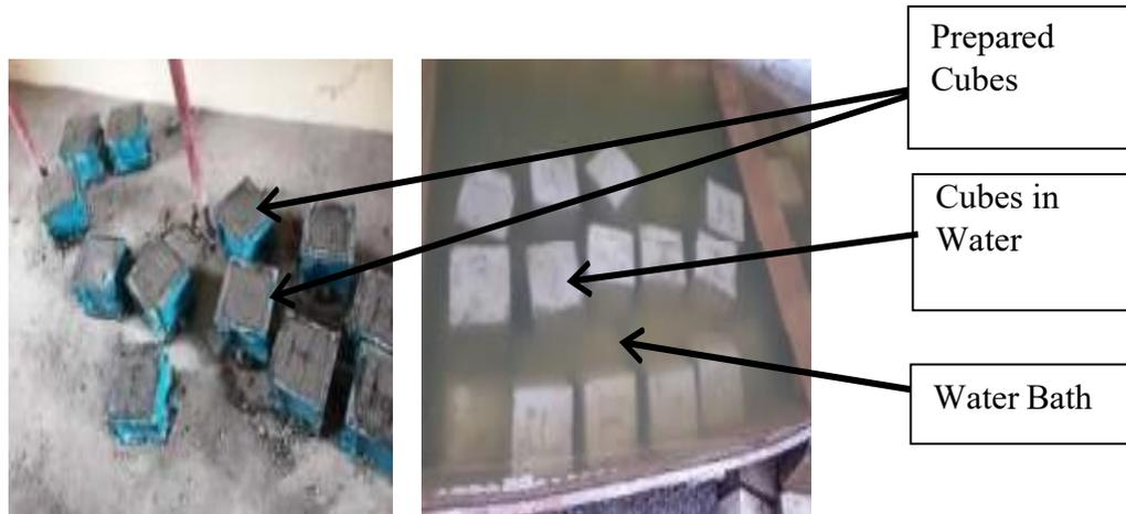
**Figure 3. 5: Concrete Cubes Cast and Cured in Water**
