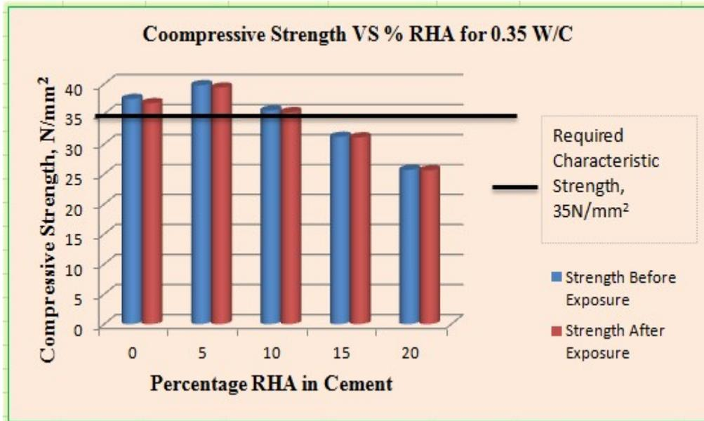
**Figure 4. 3: Compressive Strength vs % RHA in cement 0.35 W/C**
