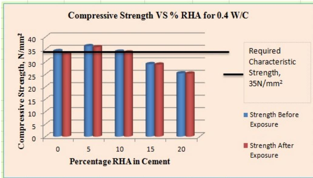
Figure 4. 2: Compressive Strength vs % RHA in cement for 0.4 W/C
