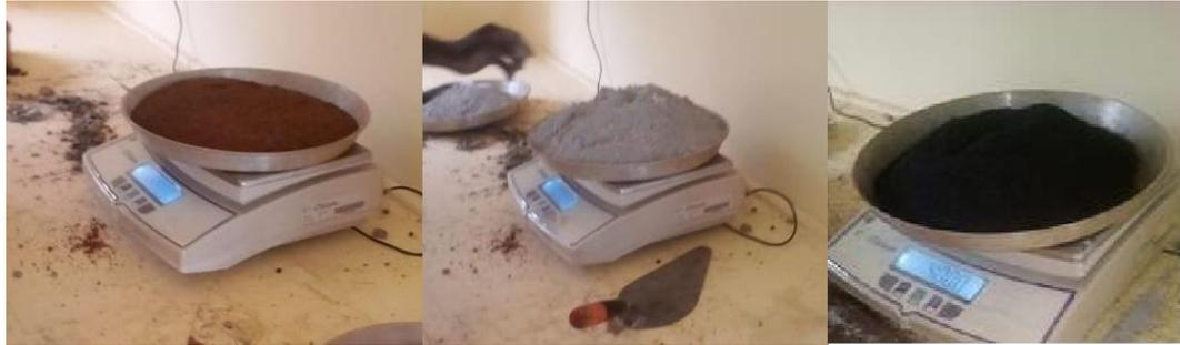
**Figure 3. 4: Batching By Weight**
