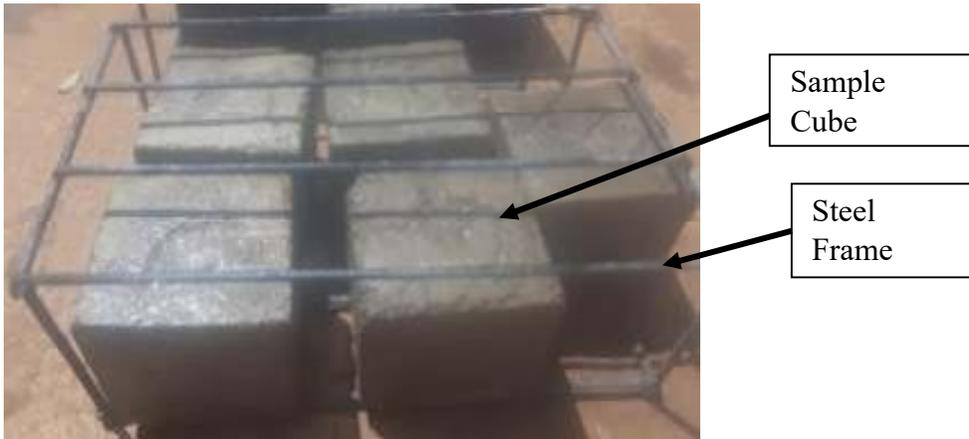
**Figure 3. 6: Samples suspended on a steel frame, ready for immersion in solution**
