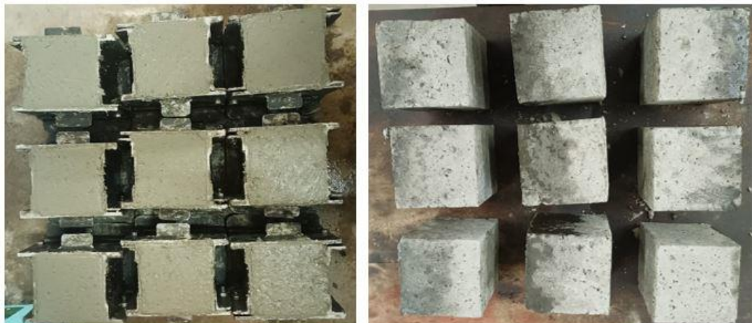
Figure 4. Fresh and Hardened Concrete Samples
