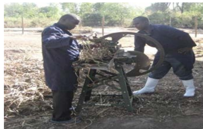
Figure 7. Chopping with a chaff cutter.
