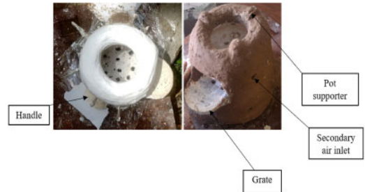
Figure 2. Stove under construction.
