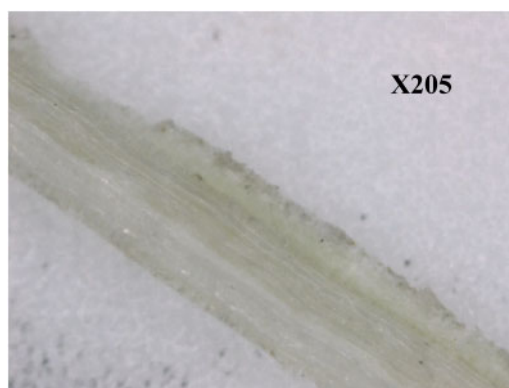
Figure 4. Micrographs of Calotropis procera bast fibres untreated taken at \times 205 .
