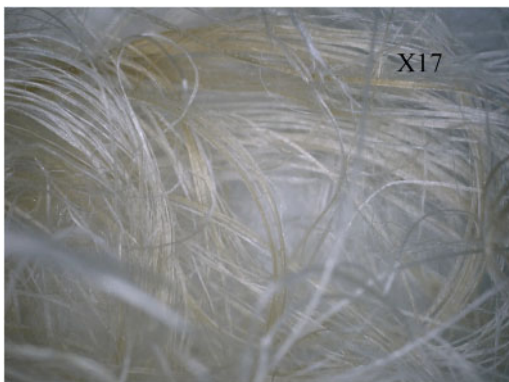
Figure 7. Micrographs of Calotropis procera bast fibres microwave-treated at 385 watts for 2 minutes taken at \times 17 .
