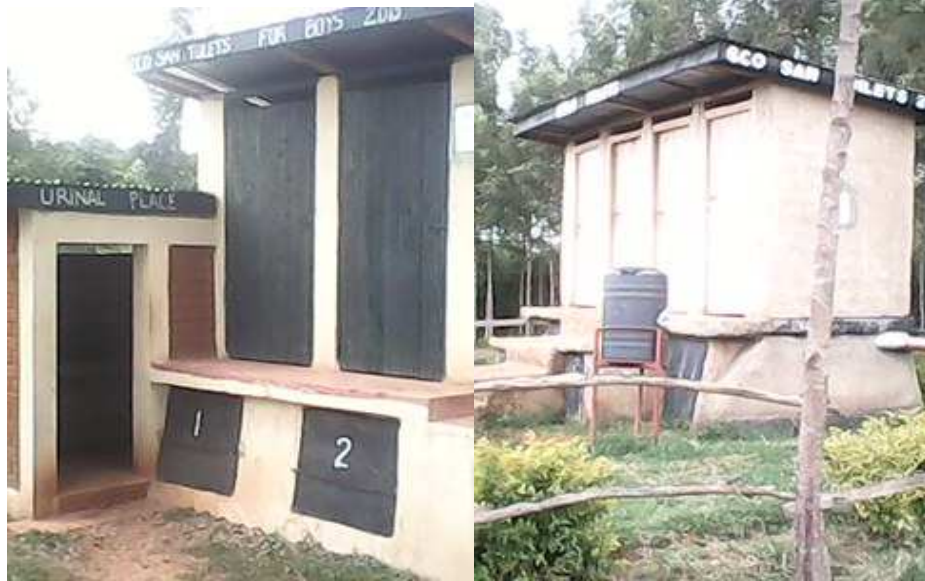
Plate 3: Eco San type of pit latrines used in some schools
