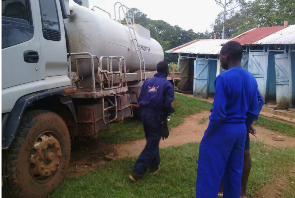
Plate 4. 4: Mechanical means of emptying pit latrines
