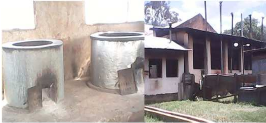
Plate 13: Improved stoves and chimneys used in secondary schools
