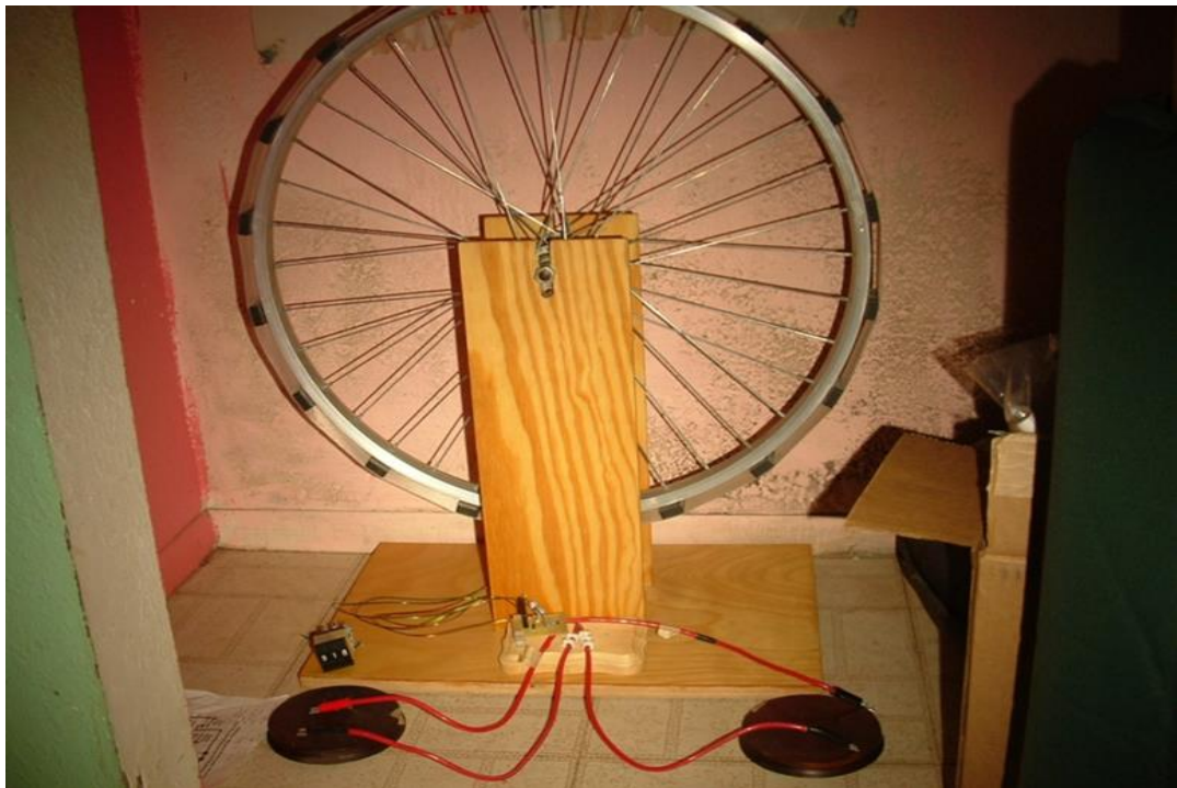
Figure 3-1: Photograph of Monopole Energizer Machine Used in The Study
