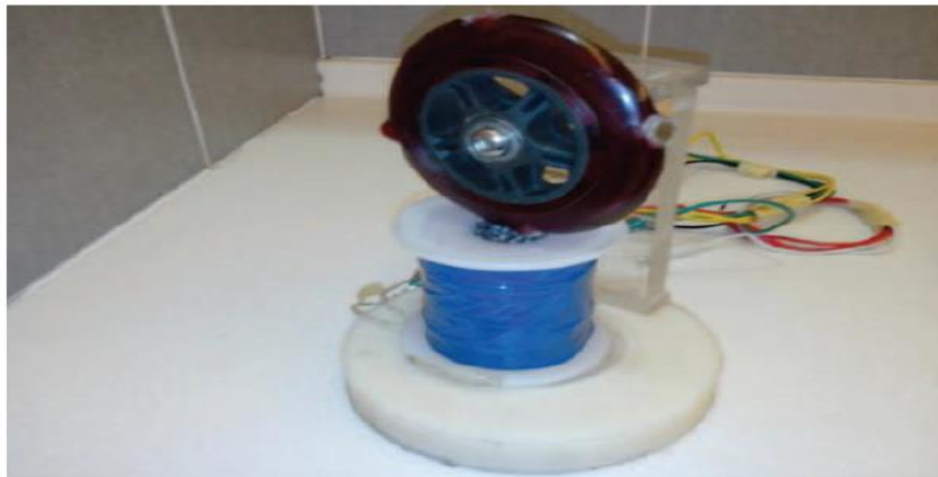
Figure 3-9: Monopole Energizer Machine Based on the Original Design (Fakhrurrazey et al., 2014).
