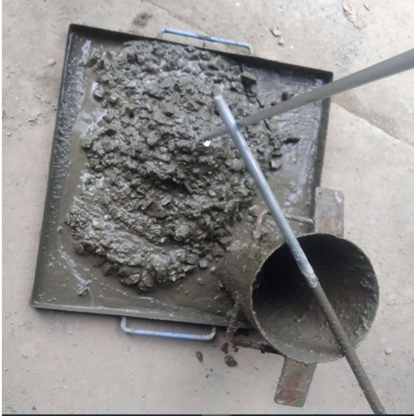
Plate 3. 3b: Slump test concrete (Collapse Slump)
