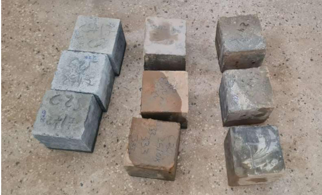
Plate 3. 5: Concrete cubes removed from a curing basin before testing for compressive strength
