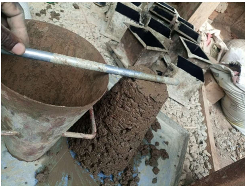
Plate 3. 2b: Slump test concrete (Zero Slump)
