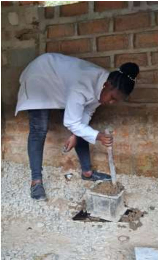
Plate 3. 4: Casting of concrete cubes
