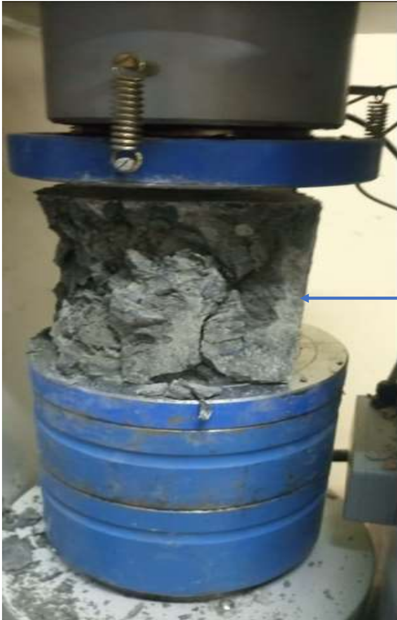
Plate 3. 6: Universal testing machine for testing the compressive strength of concrete cubes
