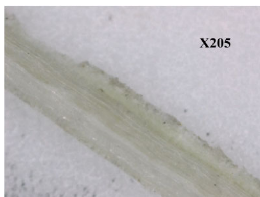
Figure 4. Micrographs of Calotropis procera bast fibres untreated taken at \times 205 .
