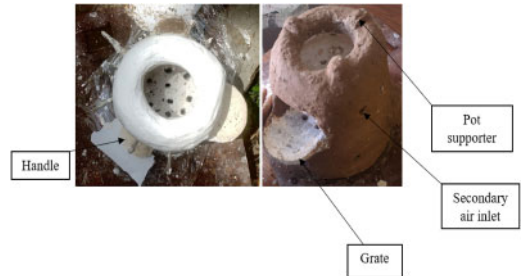
Figure 2. Stove under construction.
