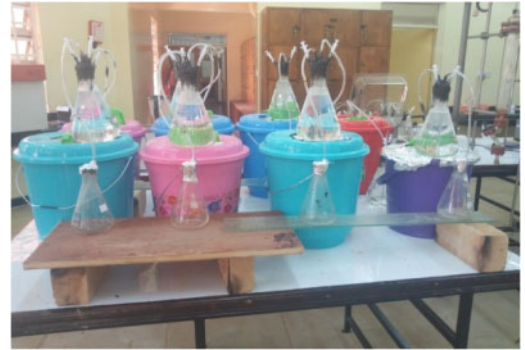
Figure 2. Full biogas set up.
