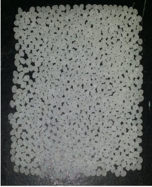
Figure 11. Poly(lactic acid) (PLA) pellets.
