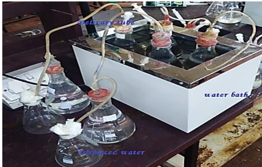
Figure 0-4: Illustration of anaerobic batch digester of maize stalk and cow dung experimental setup
