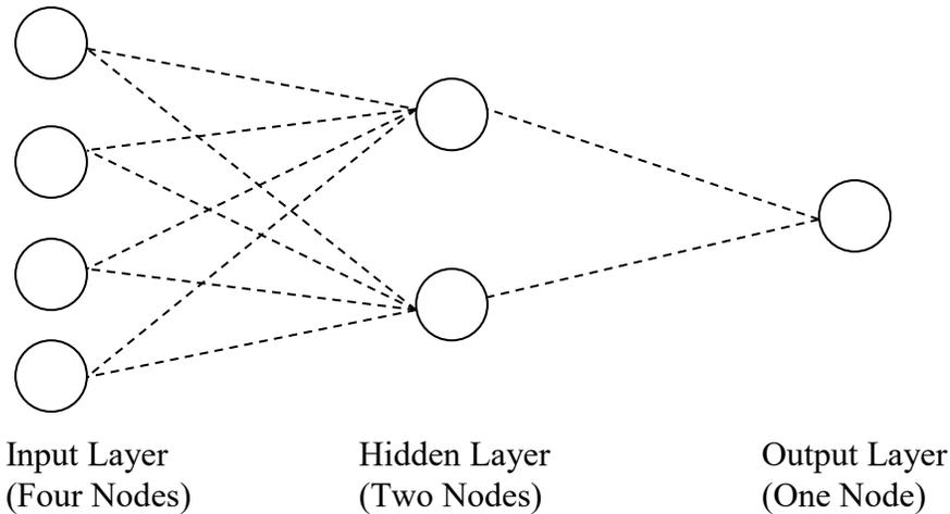
**Figure 2. 1: A typical multi-layer artificial neural network showing the input layer for four different inputs, the hidden layer and the output layer having one output.**
