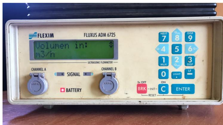
**A Clamp on Flexim Fluxus ADM 6725 Ultrasonic Flow Meter.**
