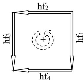
**Figure 2. 3: Part of a Network to illustrate Conservation of Energy.**
