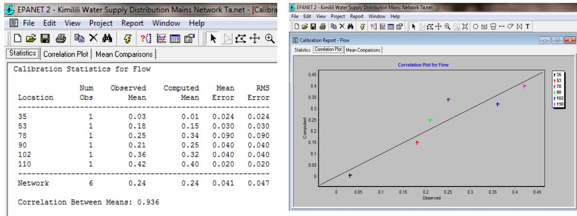
Figure 4. 12: Link Flows Calibration.
