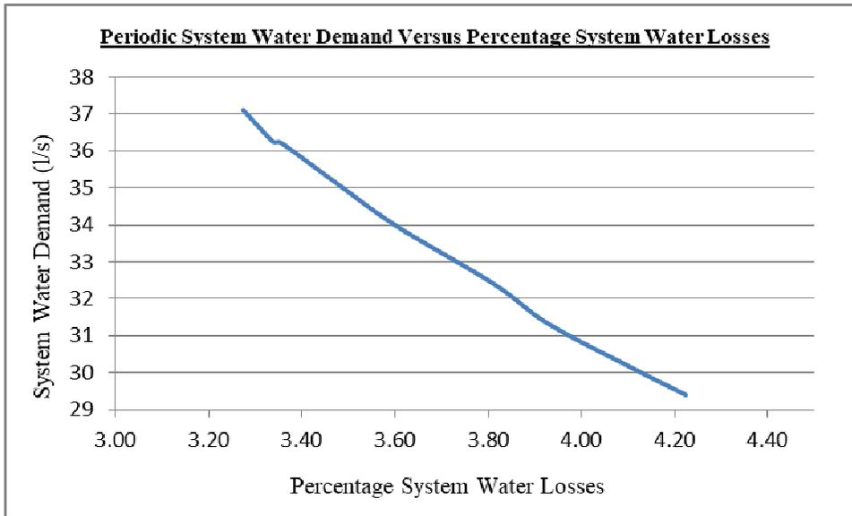
**Figure 4. 18: Periodic System Water Demand Versus Percentage System Water Losses.**
