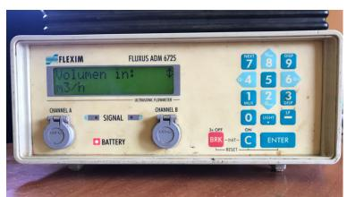
A Clamp on Flexim Fluxus ADM 6725 Ultrasonic Flow Meter.
