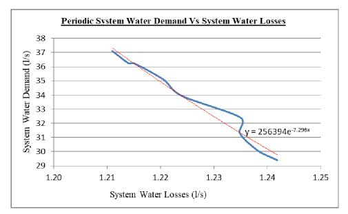
Figure 4. 17: Mathematical Relationship Between Periodic System Water Demand Versus System Water Losses.
