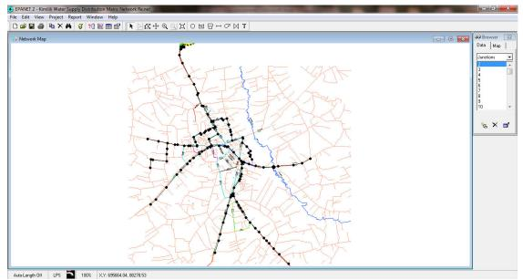
Figure 4. 9: Kimilili Water Supply EPANET 2.0 pipeline distribution network model with visible backdrop layer of distribution network.
