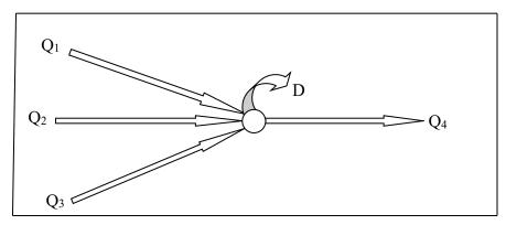
**Figure 2. 2: Continuity Equation Diagram.** Source: Oyelowo & Adeniran, (2013).
