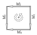
**Figure 2. 3: Part of a Network to illustrate Conservation of Energy.** Source: Oyelowo & Adeniran, (2013).
