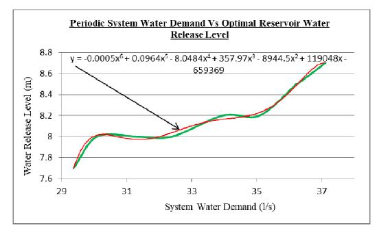
Figure 4. 21: Trendline For Mathematical Relationship Between Periodic System Water Demand and Optimal Reservoir Water Release Level.
