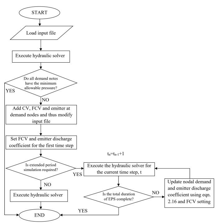
**Figure 3. 3: EPANET pressure dependent analysis algorithm flow chart.** Source: Sayyed et al, 2015
