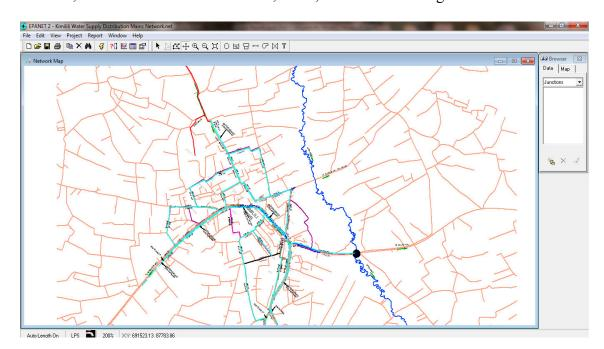
Figure 4. 8: Kimilili Water Supply EPANET 2.0 backdrop layer of distribution network.
