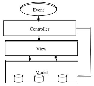
Figure 2. 1: MVC System Architecture [54]
