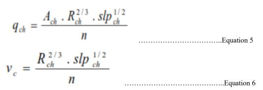
Where  $q_{ch}$  = the rate of flow in the channel (m<sup>3</sup>/s), A = the cross section area of flow in the channel (m<sup>2</sup>),  $R_{ch}$ = the hydraulic radius for a given depth of flow (m), slp = the slope along the channel length (m/m), n = Manning's coefficient for the channel and v= the flow velocity (m/s).
