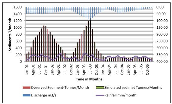
Figure 6 Calibrations for Discharge and Sediments
