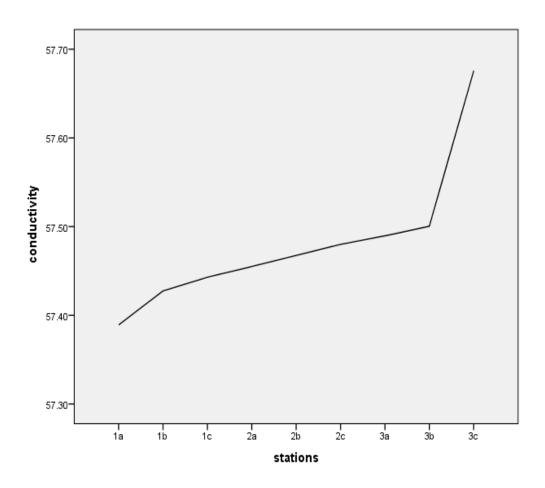
Figure 4.4: Variation in Electrical conductivity ( $\mu$ S cm<sup>-1</sup>) in River Shimiche along land use gradients.
