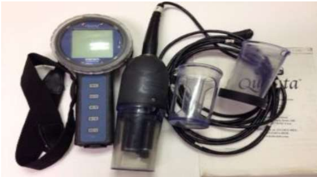
Figure 2: Quanta hydro lab water monitoring system
