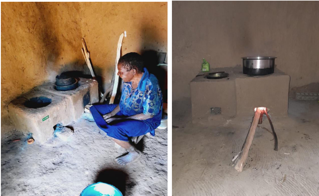
Left and Right: Twin brick rocket stove being used in the households surveyed
