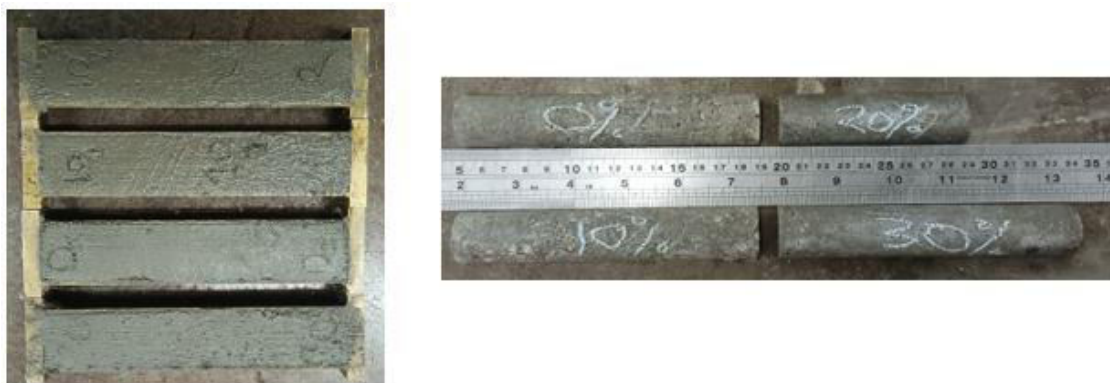
Figure 3.5: Fresh and Hardened Mortar Samples.
