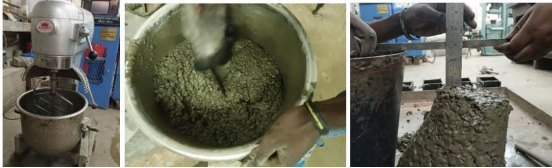
Figure 3.3: Concrete Mixing and Slump Test.
