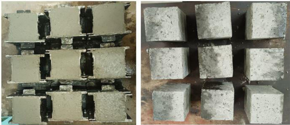
Figure 3.4: Fresh Concrete in Moulds and Hardened Demoulded Samples.
