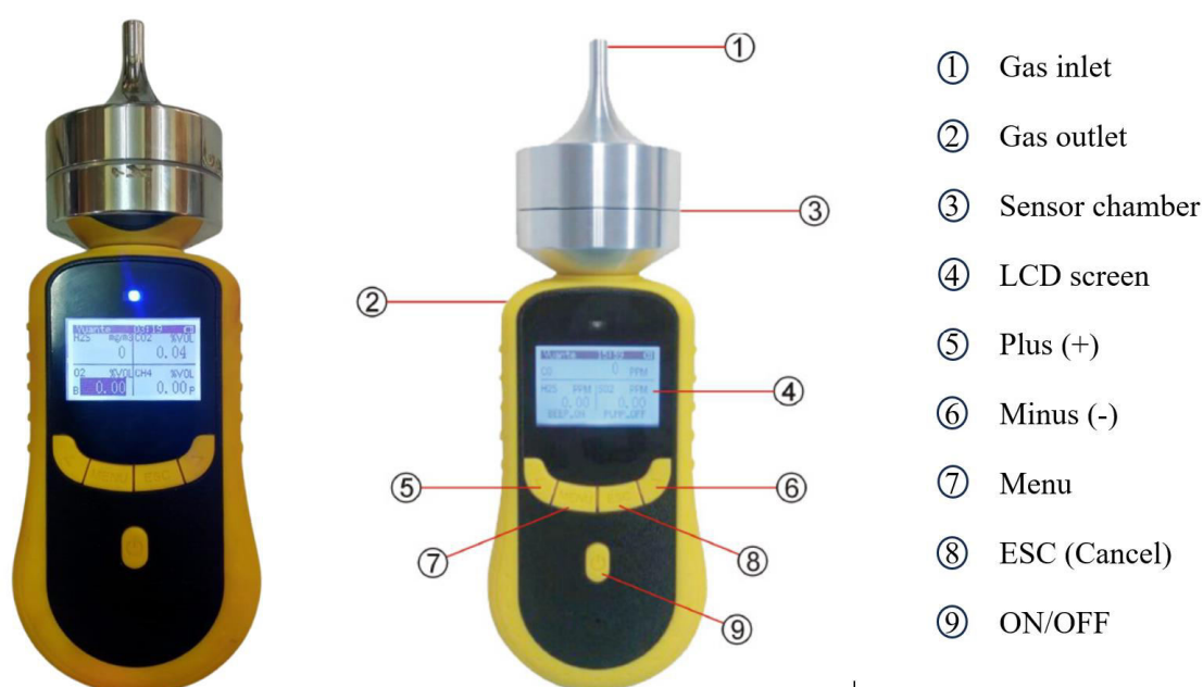
Photograph 3.2: SKY2000-M4-WH multi-gas detector; manufactured by Shenzhen Yuan Technology Co. Ltd
