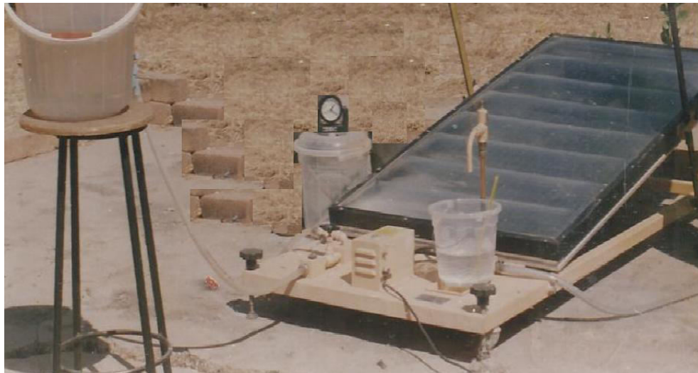
Figure 2.6: Experimental set up for Performance Evaluation of Flat Plate Solar Collector (Model Te39, (Abubakar and Egbo, 2014)
