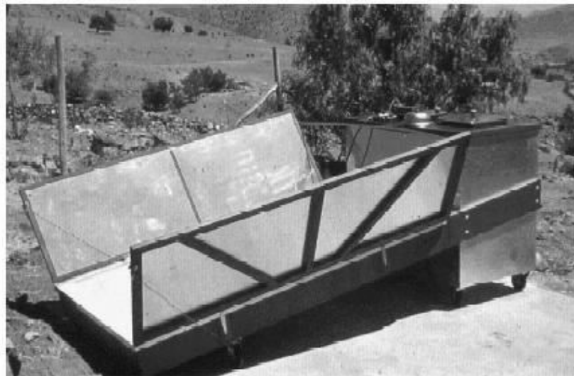
Figure 2.16: Indirect flat plate collector solar cooker with TES, (Schwarzer and DaSilva, 2003)
