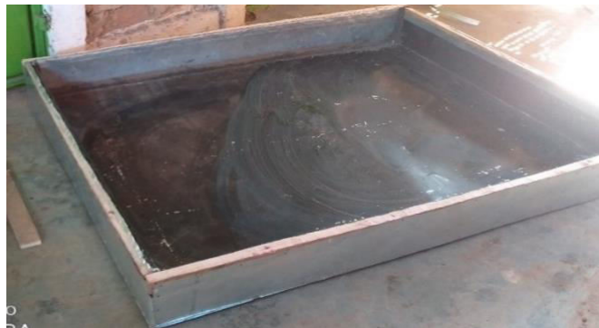
Figure 3.2: Solar collector box
