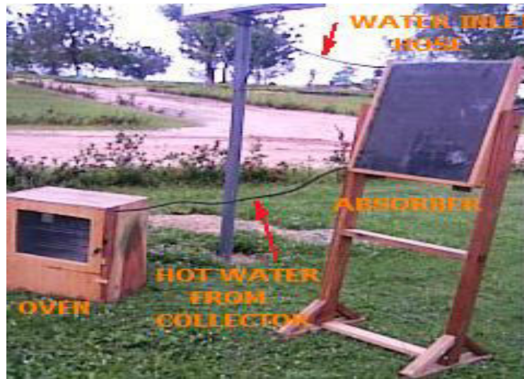
Figure 2.19: Experimental hot water solar oven set up, (Bello and Odey, 2009)
