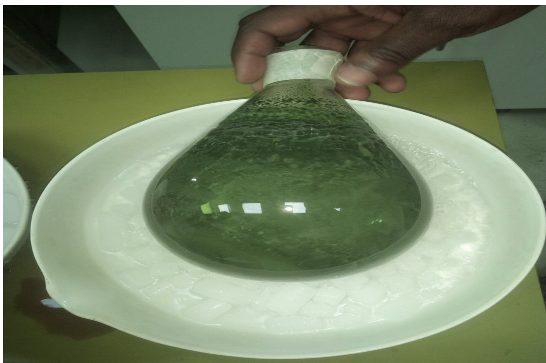
(II) Coating of Spirulina platensis filtrate with dry ice and acetone
