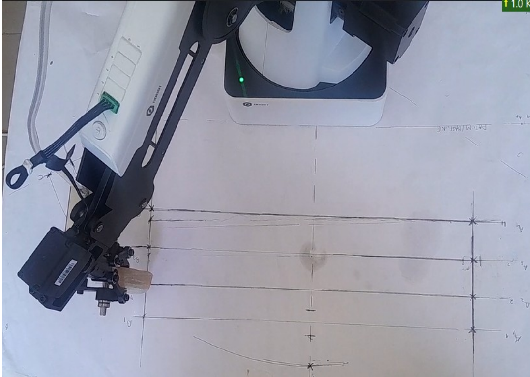
Plate Results and Discussion-15: Photograph of Dobot Magician Performing the Palletizing Task at Place point
