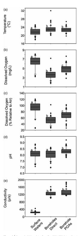
Figure 2 | Box and whisker plots of median (25%, 75% interval) water quality parameters within sites: (a) temperature, (b) dissolved oxygen (DO), (c) % DO, (d) pH and (e) electrical conductivity. Where analysis of variance (ANOVA) on ranks was significant (P < 0.05), Tukey tests were performed to determine sites that were significantly different (indicated with different letters).
